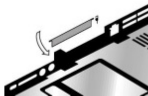
Figure 2-37. Removing a PCMCIA Door
